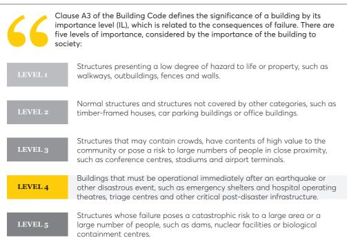
The required level of seismic performance increases with each level of importance. In general, important structures, such as hospitals, communications centres and those that provide occupation for many people, are designed for a greater level of earthquake shaking than ordinary commercial structures.
