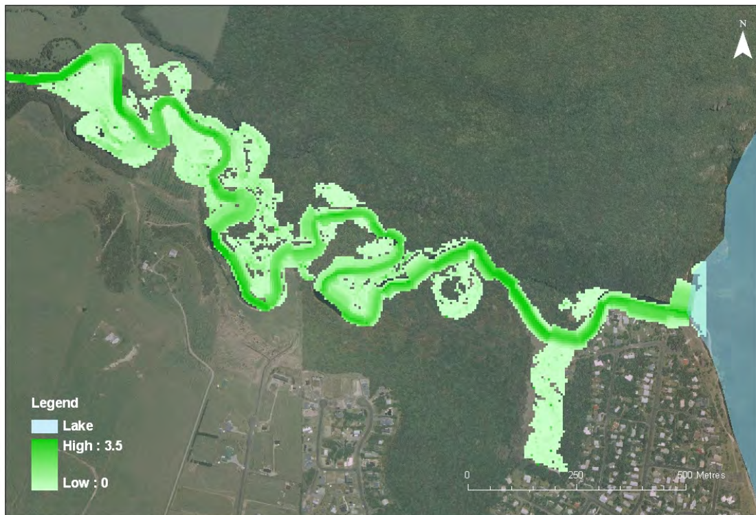
Figure 7.3: Water velocity during the 100-year flood event in the Kuratau River allowing for the effects of climate change on runoff within the catchment. Lake level is assumed to be at 357.5m.
