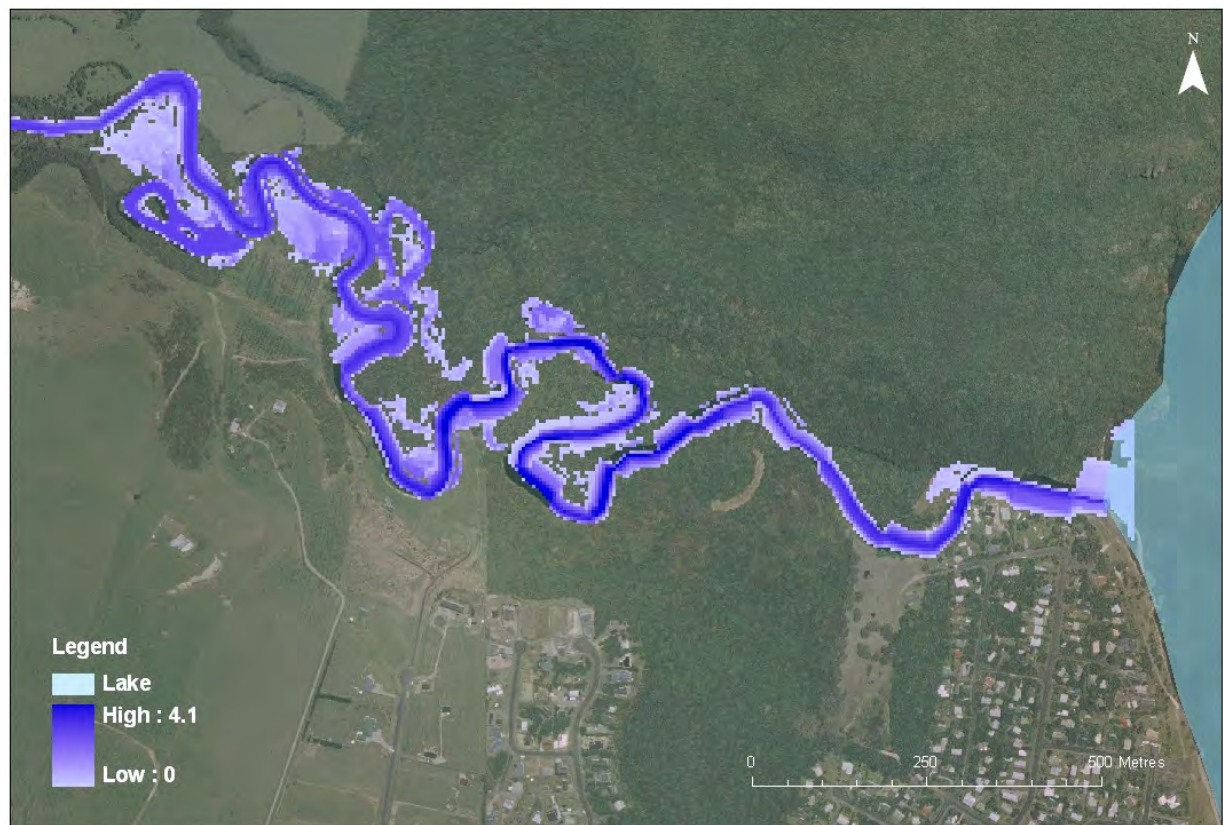
Figure 6.2: Predicted flood extent during the 29 February 2004 event using the calibrated MIKE21 model.
