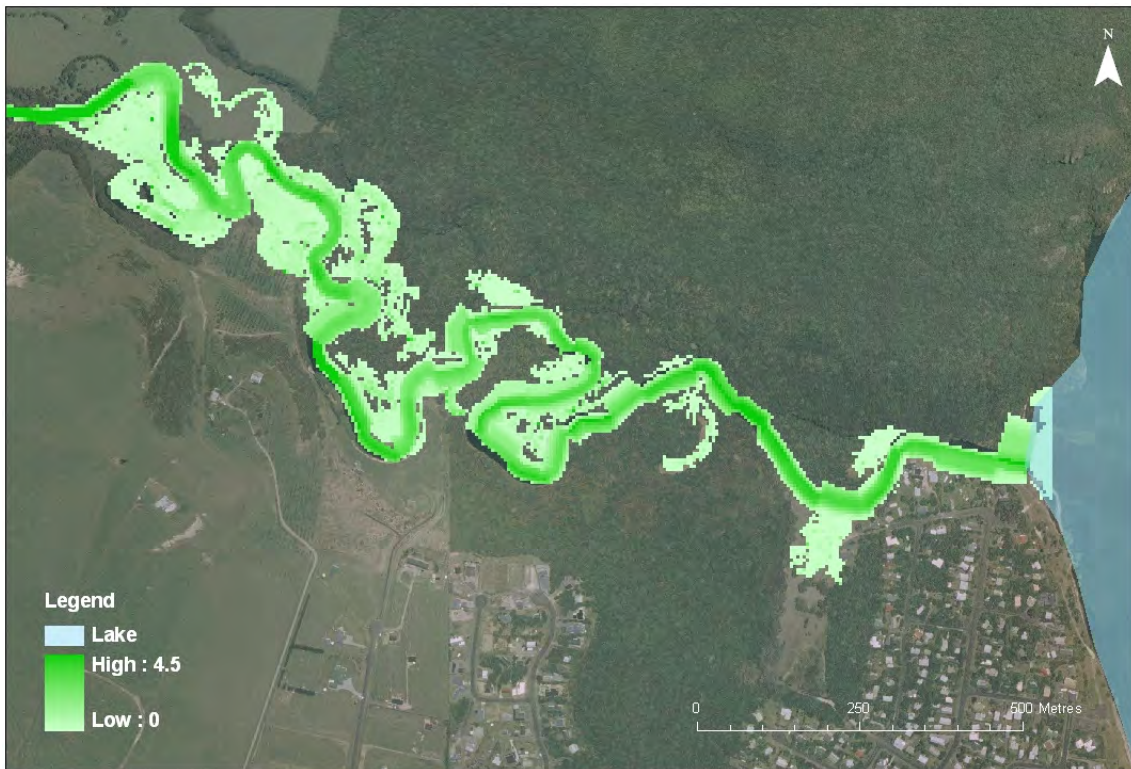
Figure 6.7: Velocity of flood waters predicted for the 100-year flood event and a lake level of 357.5m.
