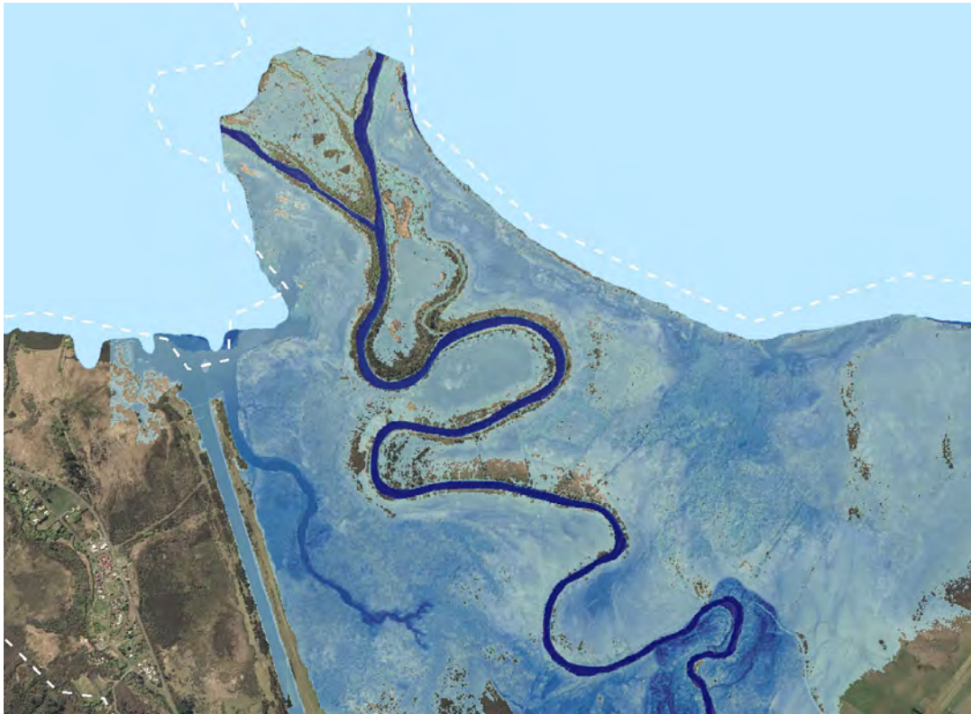
Figure 5.1: Area likely to be affected by the 100-year flood in the Tongariro River, predicted from the instrumental record and assuming a lake level of 357.5m.
