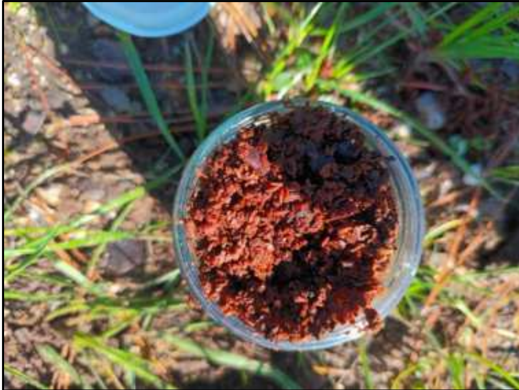
Photograph 13: Buried sawdust in the north and east of the earthwork area.
