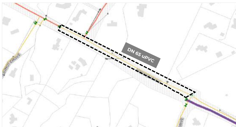
Figure 19 - Mapara Road (middle) - Existing Pipe Sizes
