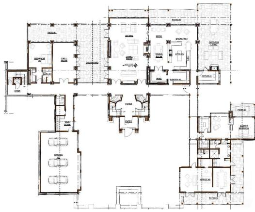
Image 15: Main Level Floor Plan
