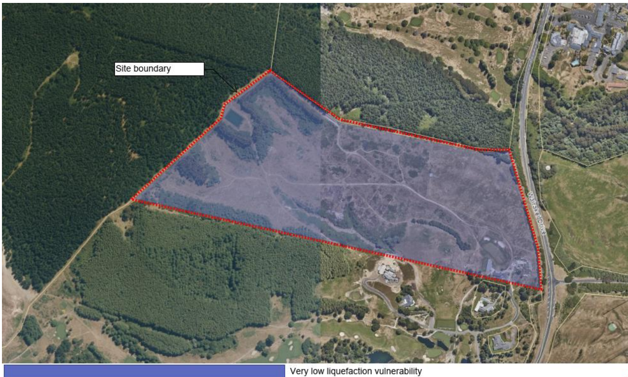
Figure 6-1: Preliminary liquefaction vulnerability map
