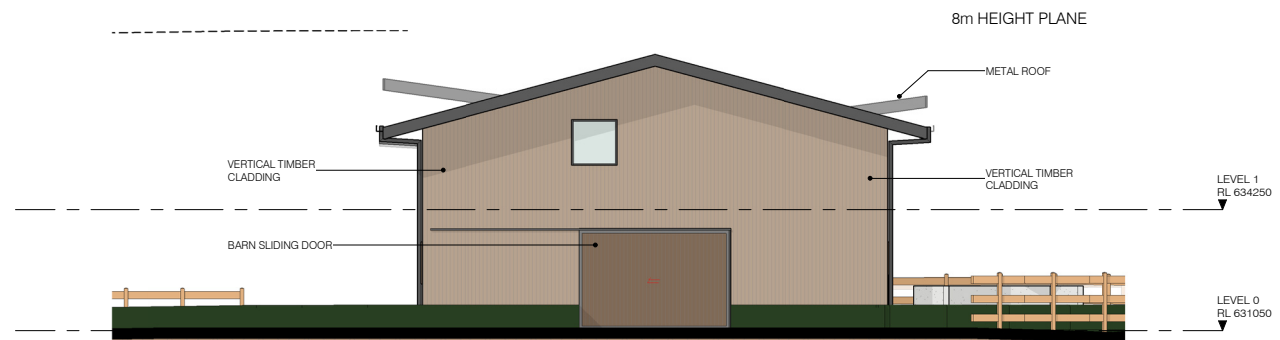
4 STABLES - NORTH EAST ELEVATION A005 1:100 @ A1 1:200 @ A3
