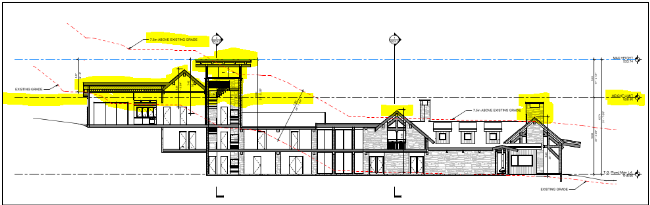
Figure 6: Section through Proposed Dwelling
