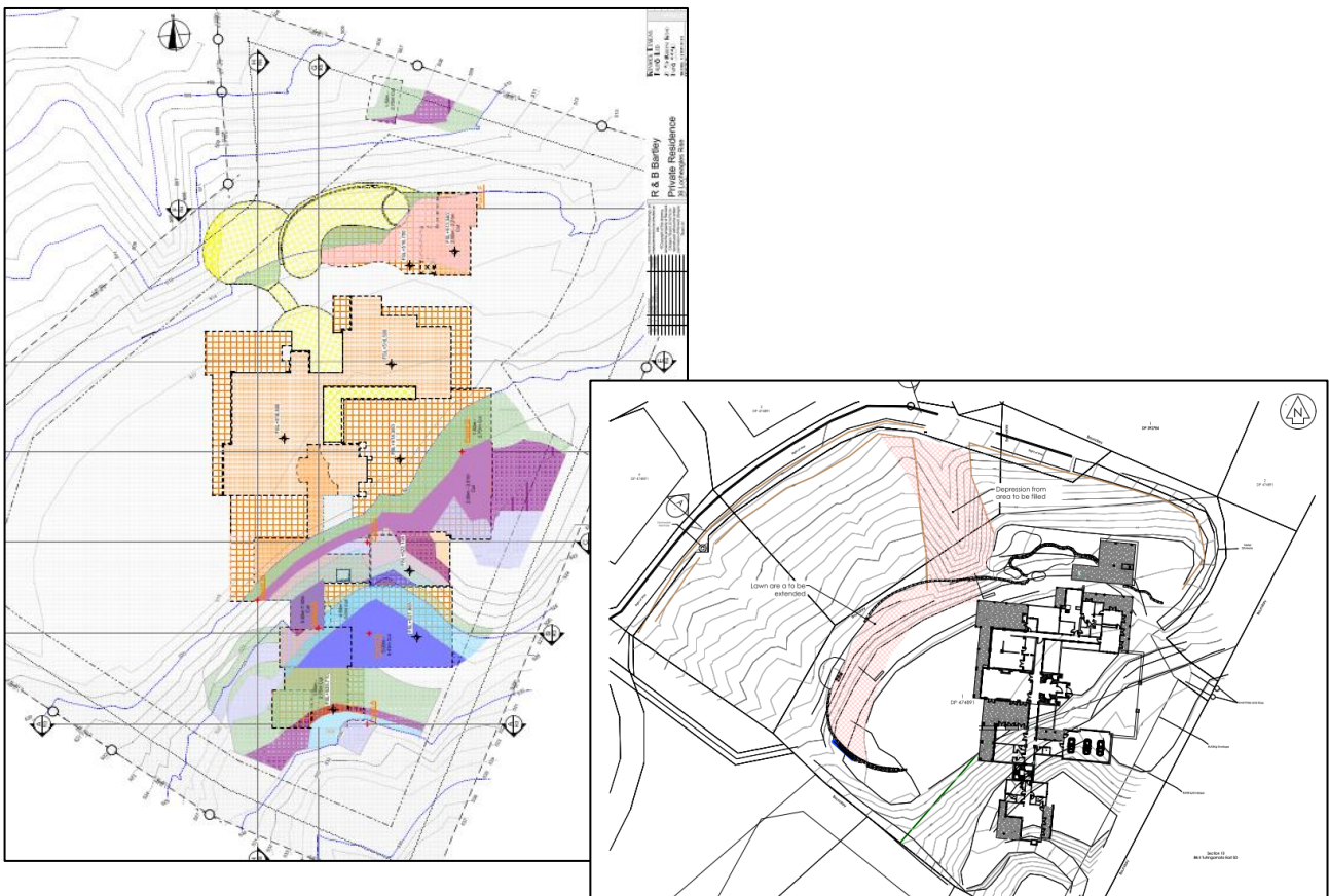
Figure 8: Earthworks Cut/Fill Plan & Fill Plan
