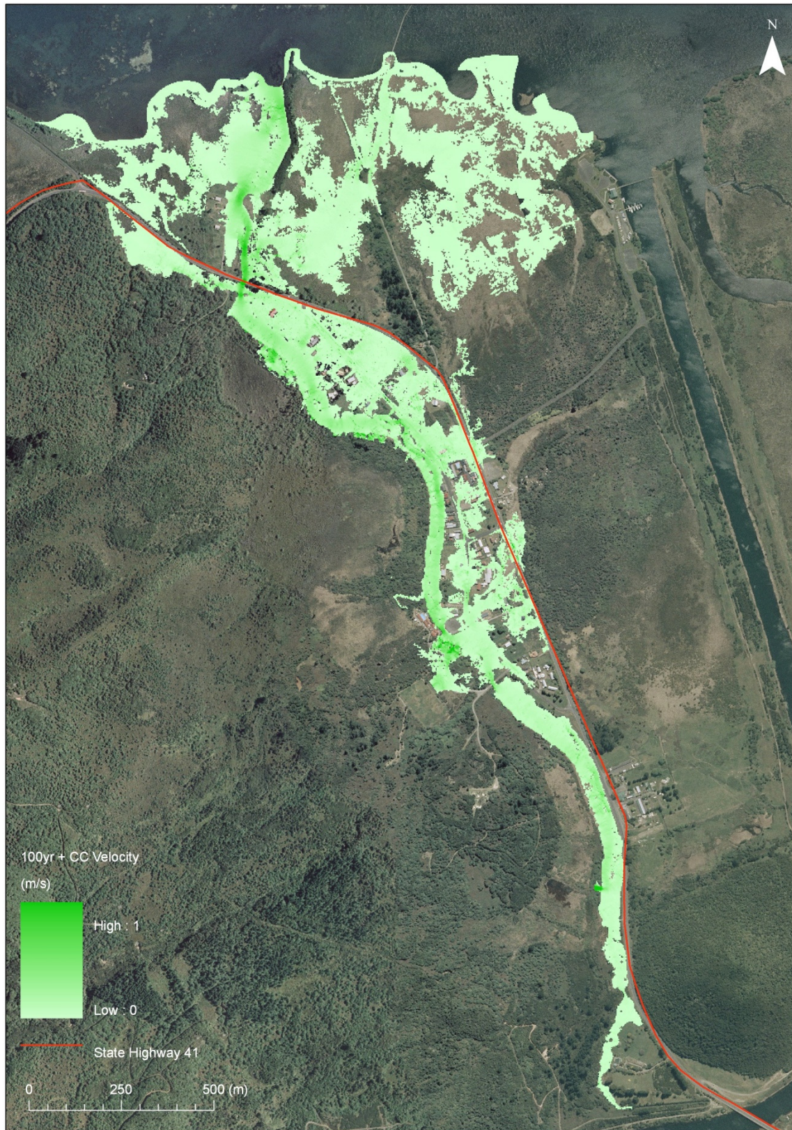
Figure 6.5: Flow velocity of flood waters in Tokaanu Stream; assuming a ‘worst case’ scenario i.e., 100-year flood event increased to allow for the predicted effects of climate change and a lake level of 357.5m.
