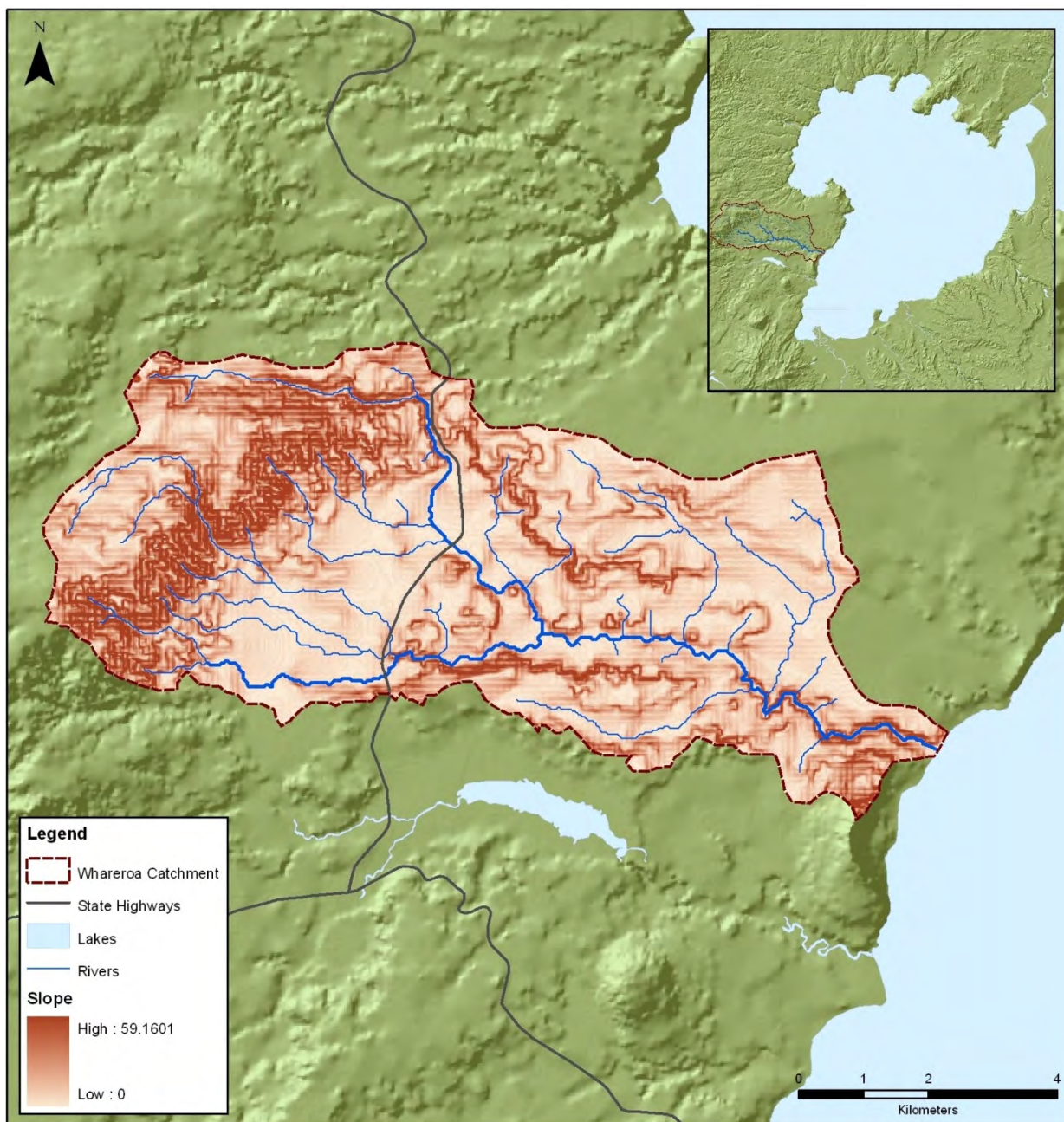
Figure 2.4: Slope within the Whareroa catchment.
