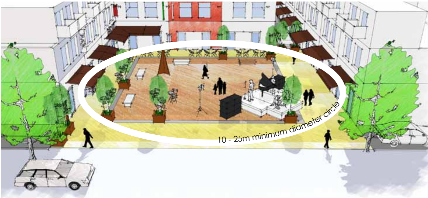
Getting the scale of squares and plaza right is critical. While horizontal proportions need to relate to the scale of surrounding buildings, the minimum dimensions shown above enable multiple uses to occur. ✅
