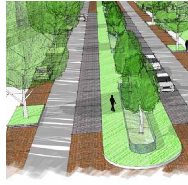
Narrower carriageways, delineated parking zones and planting help to create a slow-speed, shared street environment. ✓
